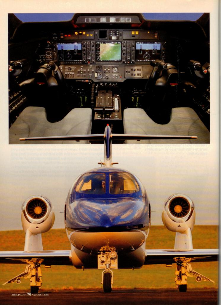
minum fuselage with frames and stringers, except the components are made of composite materials. The cockpit and tail section is a honeycombsandwich construction to maintain the compound curves, which are especially important for the laminar-flow nose. The sandwich and stiffened panels are co-cured in an autoclave to reduce weight and cost. Normally, such materials would need to be cured separately and then mated, but Honda developed a method whereby they can be cured at the same time.
